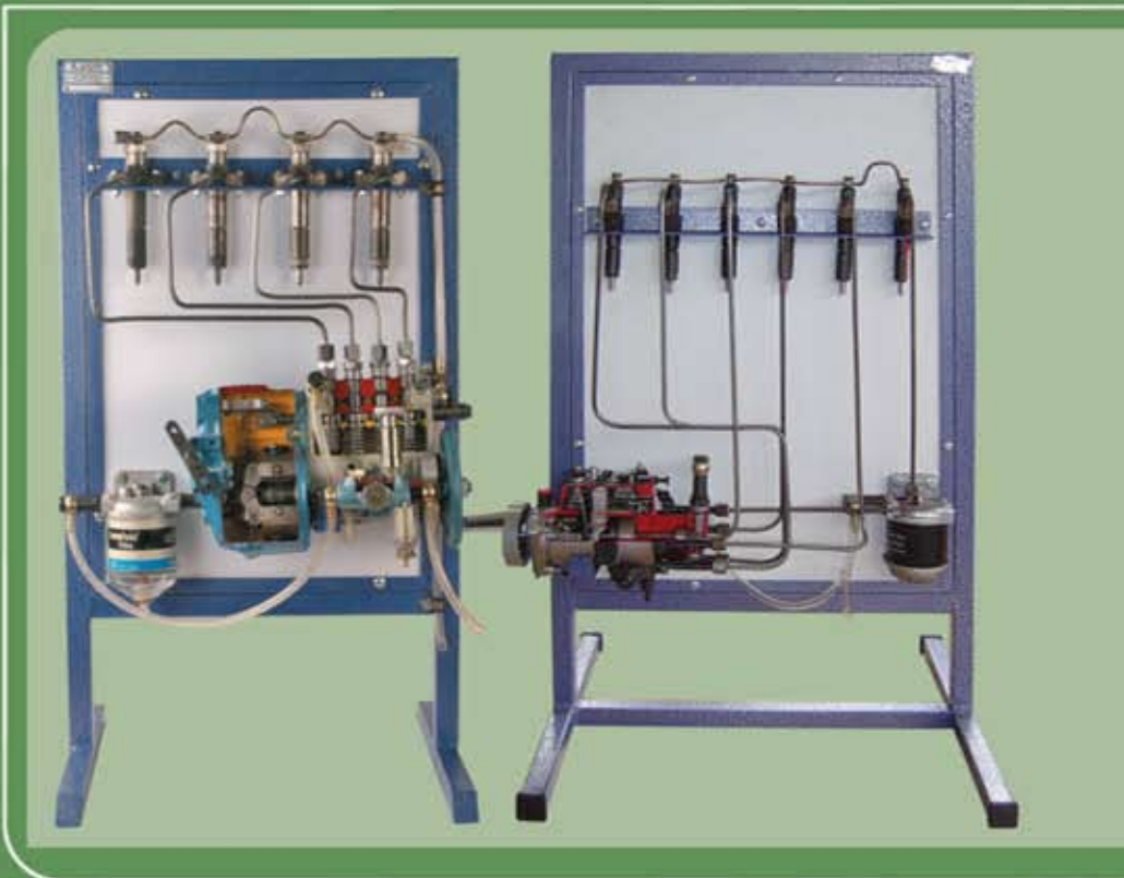
4-unit lined injection pump panel with fuel filter and injections
