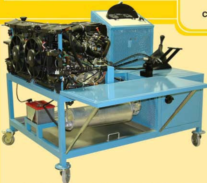
Set of injection motor of Peugeot 405 with its power transmission system
