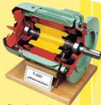
Sectioned induction motor
