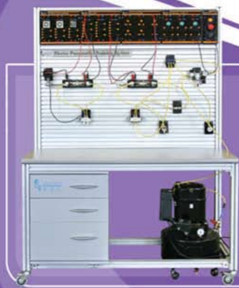
Electro hydraulics with PLC set
